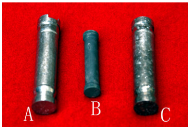
Fig. 1. Samples after HIP processing. (A) W–Zr sample, at 1300 °C, (B) W–S.S. sample, at 1200 °C, (C) W–Zr sample, at 1400 °C.
